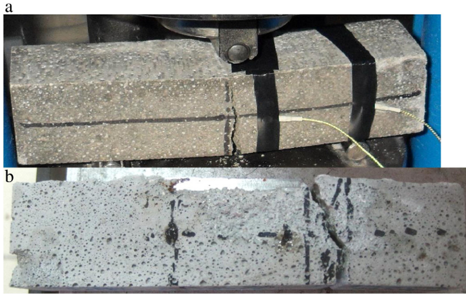
Fig. 5. Fractured specimens after (a) bending, and (b) shear.
